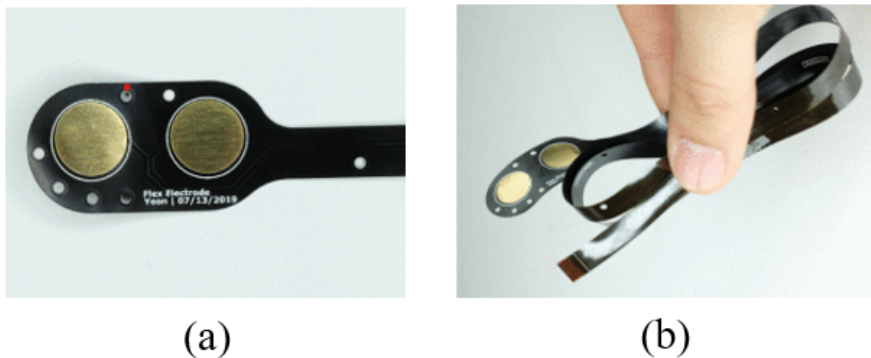
Figure 2.4. Manufactured electrode proposed by Yeon et al. (a) Close up on the electrode developed electrode. (b) Illustration of the electrode's flexibility post-production.
