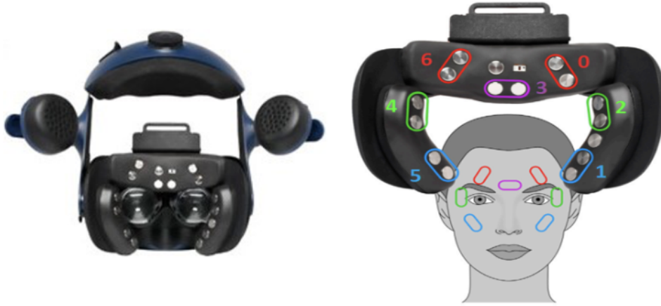
Figure 2.2. EmteqPRO™ multi-sensor face mask employed in the study conducted by Kiprijanovska et al [43].
