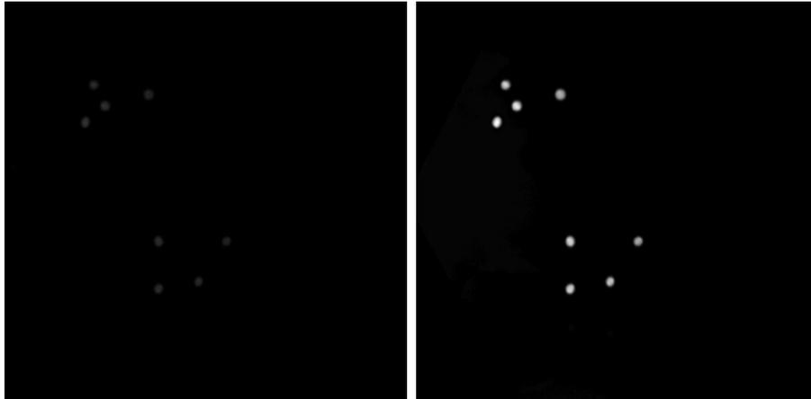
**Figure 2.10:** Raw Image from IR camera. On the right image with enhanced contrast
