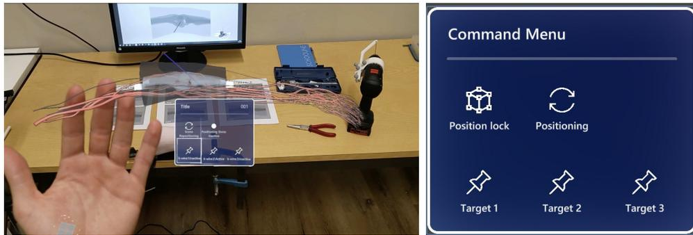
**Figure 3.6:** Command Menu displayed in AR user interface
