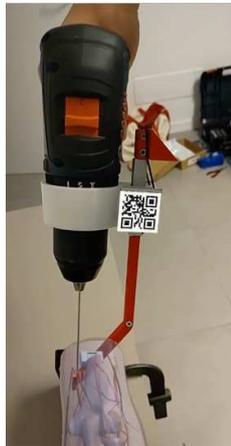
**Figure 6.3:** QR tracking and models superimposition
