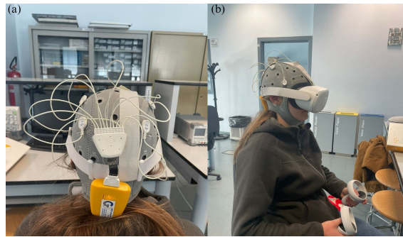
Figure 5.2. Illustration of the Assembly of the EEG System and the Oculus on the User: (a) Rear View; (b) Side View.
