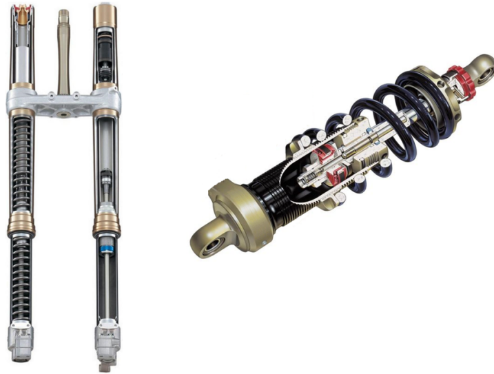
Figure 4: Common suspension layout for motorcycle applications. Left: Front suspension assembly. Right: Rear suspension assembly
