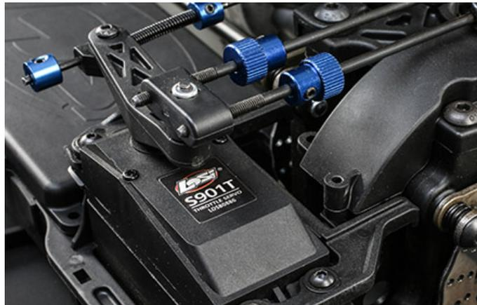
Figure 2: Throttle servo motor of Losi 5IVE-T 2.0.
