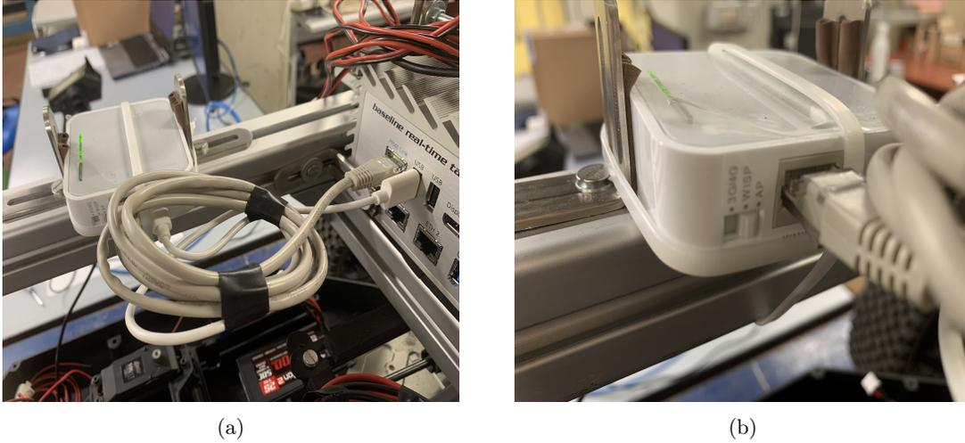
Figure 23: TP-LINK TL-MR3020 router interfaces.
