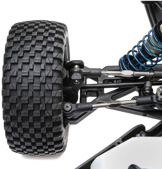
Figure 3: Part of Ackermann adjustable system of Losi 5IVE-T 2.0.
