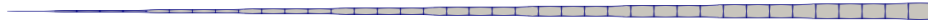
Figure 5.1.2: Slice of the pipe discretized with a relatively refined mesh having y^+ falling in the log-law region.
