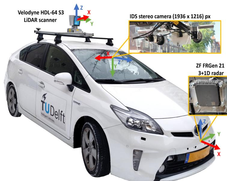
Figure 3.2: Car setup in View of Delft [49]
