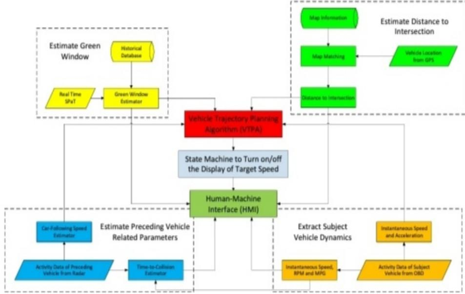
Figure 2.2: EAD System Architecture [8].
