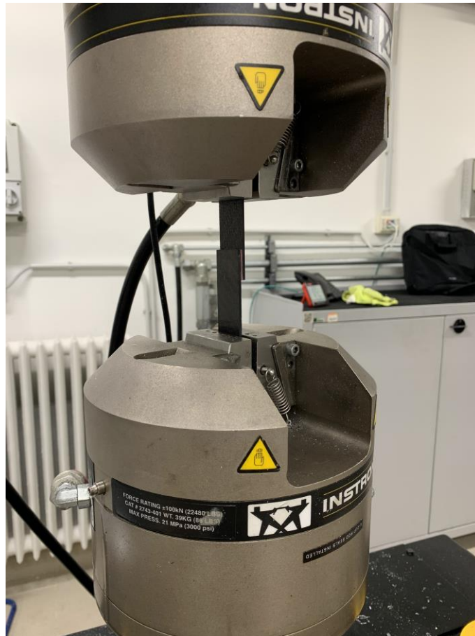
Figure 39. SLJ tested specimen
