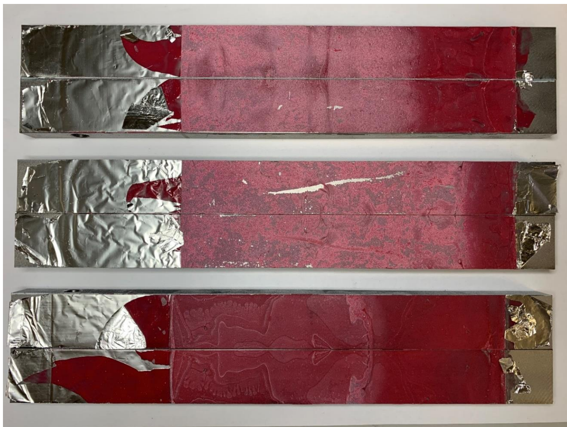
Figure 28. Fracture surfaces T0.3 (A – C – B)
