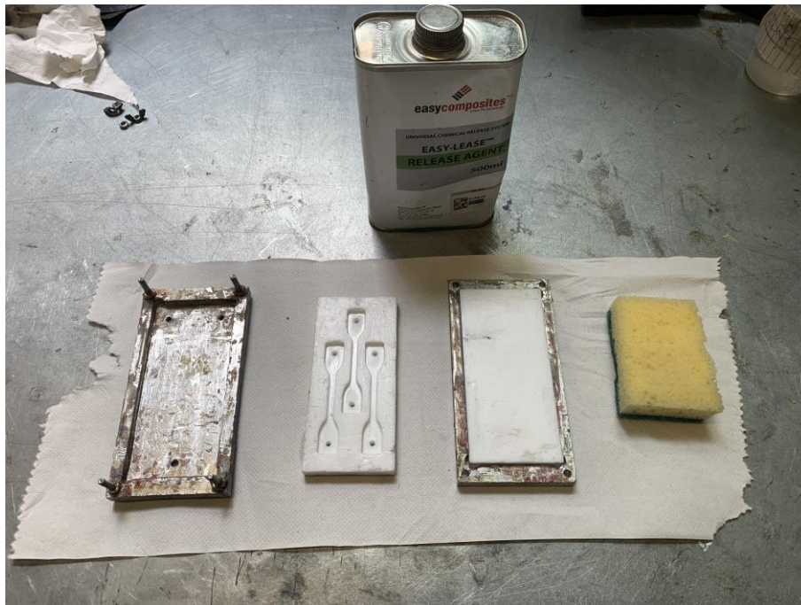
Figure 13. Release agent application on Teflon die
