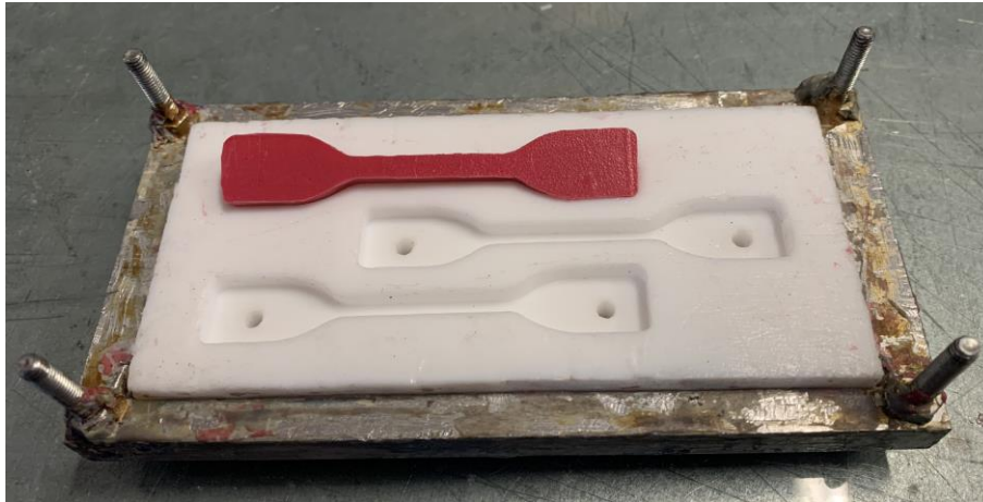
Figure 14. Teflon die with cured specimen
