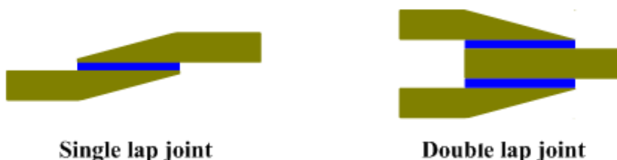
Figure 8. Single and double lap joint [6].
