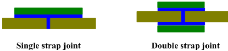
Figure 9. Single and double strap joint [6].
