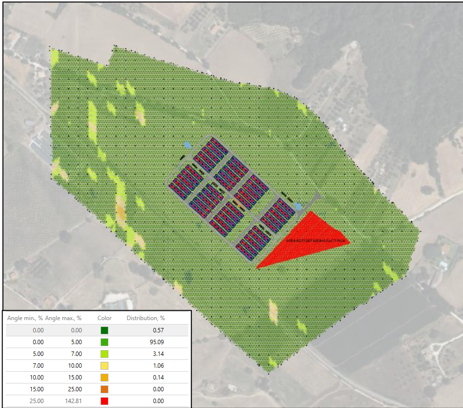
Figure 31: BESS plant slopes (E-W direction)
