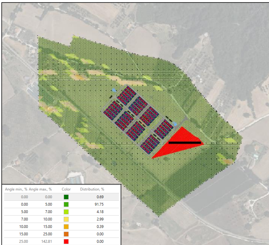
Figure 32: BESS plant slopes (N-S direction)
