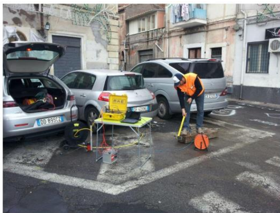
Figure 2-4 Typical configuration used in down-hole seismic testing and Site Application
