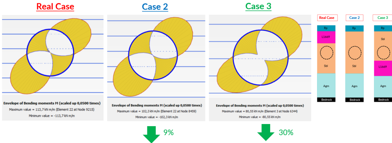
Figure 5-28 Envelope Bending Momen kNm/m – Non-Slip Condition
