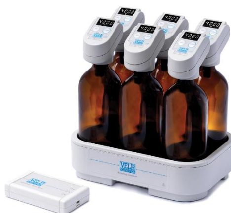
Figure 13: Respirometric sensor System [30].
