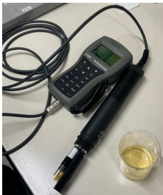
Figure 17: Multiparametric probe used for the analysis of the leachate.
