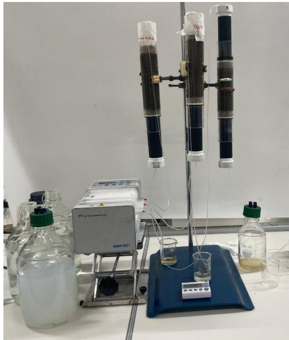
Figure 16: Organization of the column setup: it is organized as the test done in summer, without the spectrophotometer.
