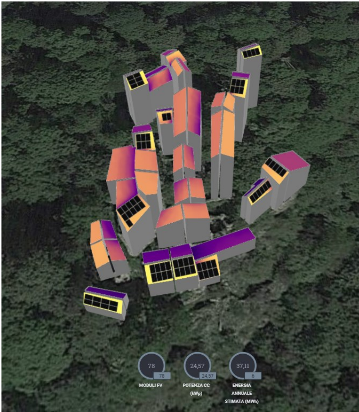
Figure 32 SolarEdge estimation considering Aleo Solar S_79 SOL-T panels [73]
