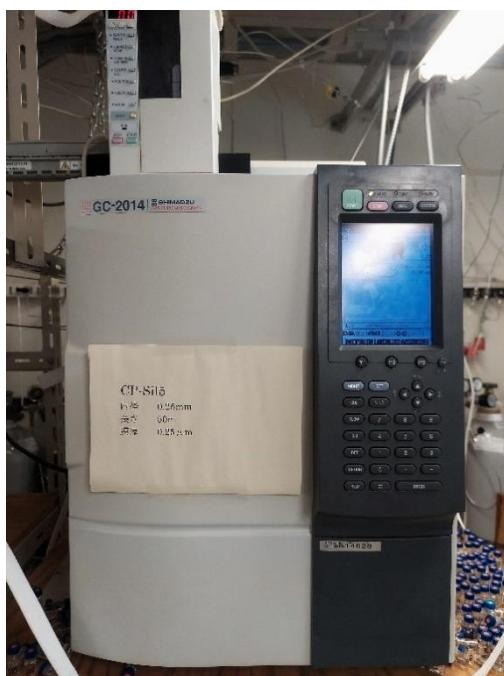
**Figure 21** - Gas chromatograph *Shimadzu GC-2014*
