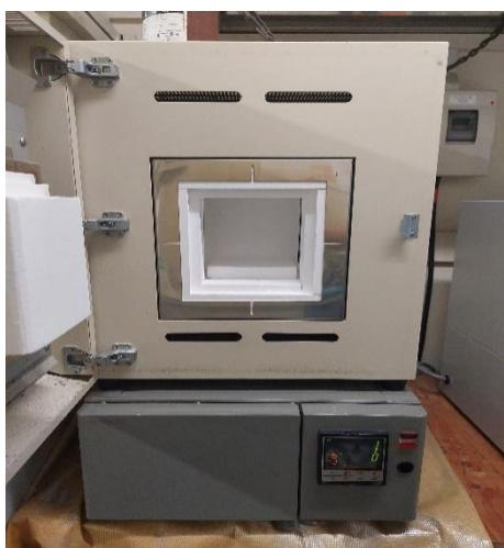
**Figure 19** - Electric furnace *Advantec FUH312PB*
