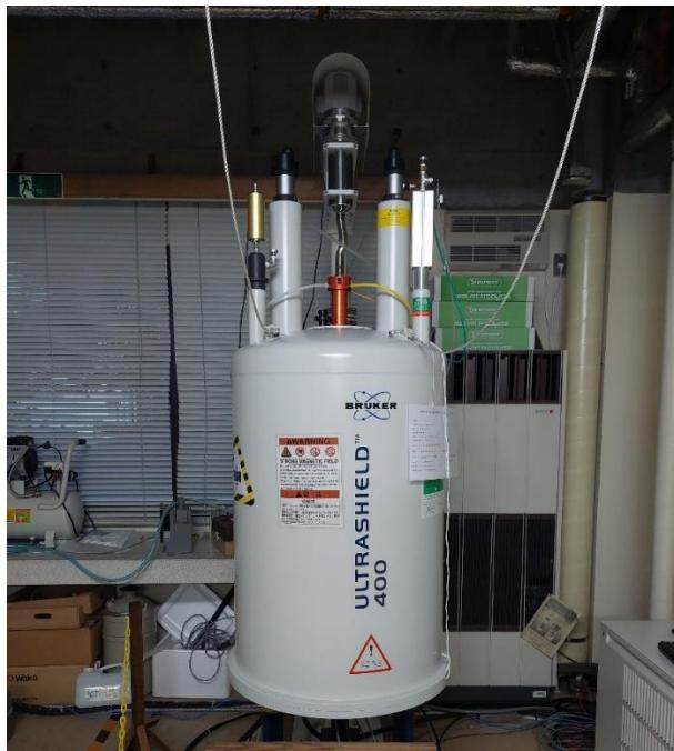
**Figure 23** - NMR spectrometer *Bruker Ultrashield 400*
