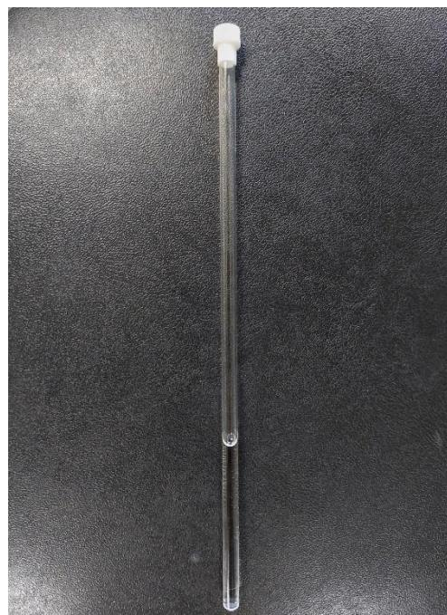
**Figure 28** - Sample for NMR spectrometry
