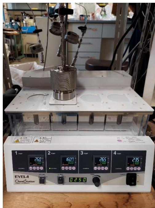
Figure 25 - EYELA ChemiStation Personal Synthetizer PPV
