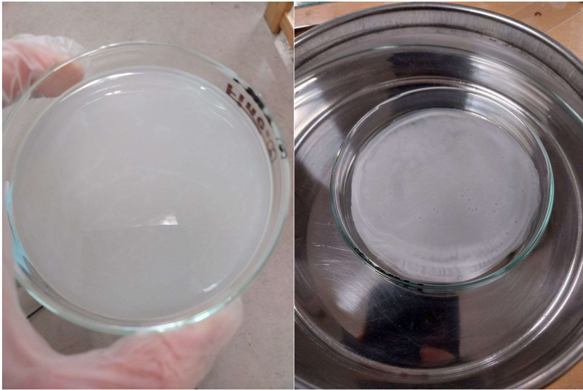
Figure 15: Images of the cast composite solution before and after drying at room temperature and pressure
