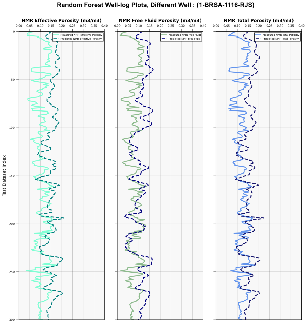
Figure 4-16: Comparing the match between the predicted and measured NMR porosity, for the RF Model, applied to the different well (1-BRSA-1116-RJS): Left track: Predicted and Measured NMR Effective Porosity (m 3 /m 3 ). Middle track: Predicted and Measured NMR Free Fluid (m 3 /m 3 ). Right track: Predicted and Measured NMR Total Porosity (m 3 /m 3 ).
