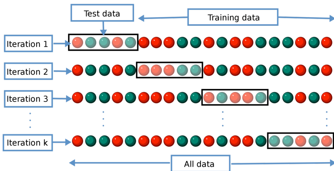
Figure 3-1: K-Fold Cross Validation Concept with K iterations across the Test & Train datasets
