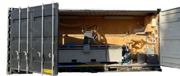
Fig.110. Mobile Production Facility (MPF) del sistema D-Process Facit Homes. Fonte: https://www.facit-technologies.com/mobile-production
