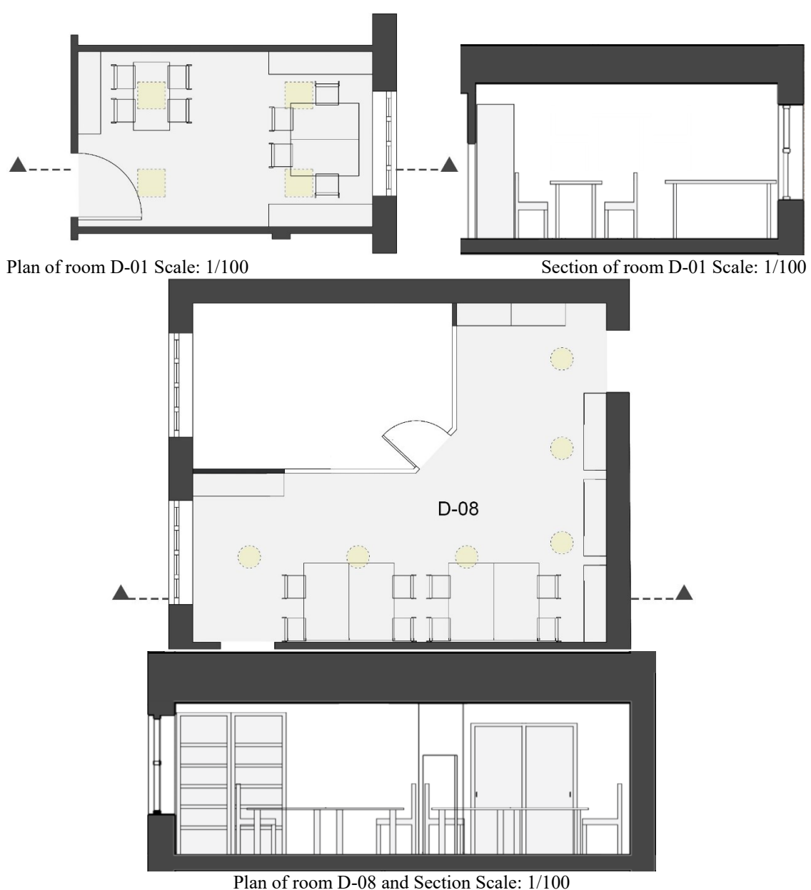
Figure 8.17. Plans and sections of rooms D-01, and D-08 with artificial lightings and furniture
