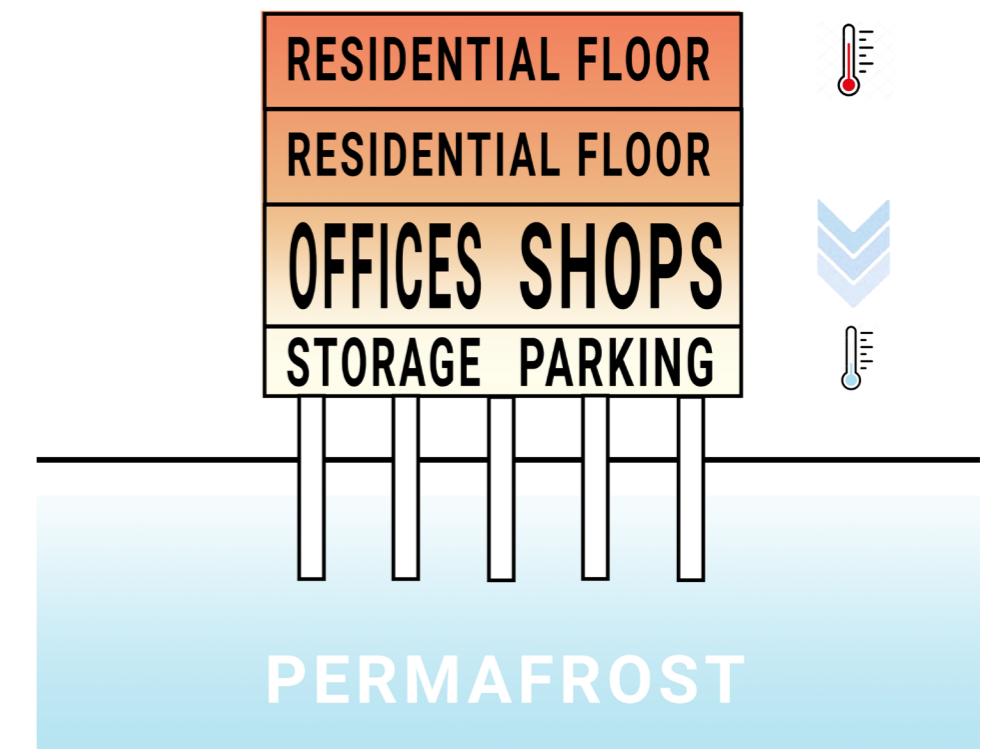
Figure 68 (on the right): a scheme shows how it is possible to reduce the effect of the building on permafrost by design. Placing the different functions of the building according to their temperature requirements. The hottest areas, like residential blocks, should be placed on top, as further as possible from the ground. The coldest, like storage rooms and parking, have to be placed close to the permafrost. In this way, the hottest areas will transfer heat not to the ground but to the storage area and parking, so in the end permafrost will receive less heat than if the building was fully residential
