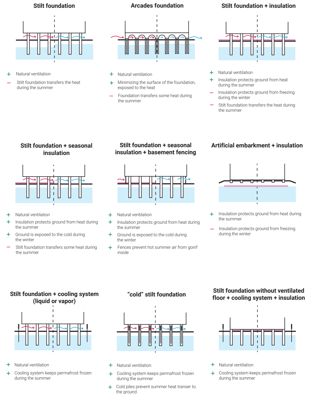
Figure 62: Scheme shows different solutions of the foundation for the buildings for the permafrost regions and its advantages and disadvantages
