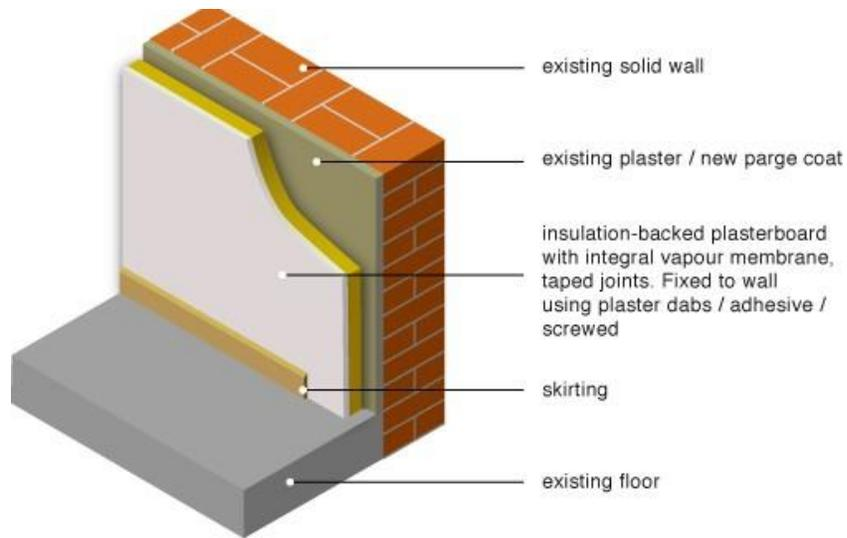
Fig 8. Insulation of internal walls with insulated plasterboard. (Source: [www.greenspec.co.uk](http://www.greenspec.co.uk) building design), (Chinazzo, 2013-14)
