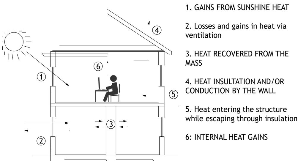
Fig 40. Heat flow diagram in a building. (Chinazzo, 2013-14).
