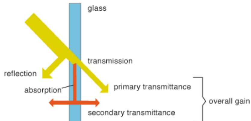
Fig 20. Solar gains through windows (Source: [www.greenspec.co.uk buildingdesign](http://www.greenspec.co.uk/buildingdesign)).
