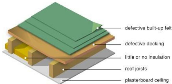
Fig 18. Cold roof insulation (Source: [www.greenspec.co.uk](http://www.greenspec.co.uk) building design).
