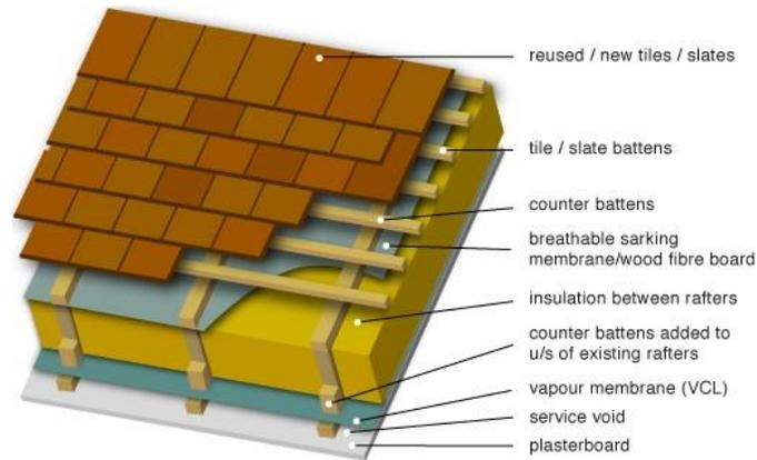
Fig 13. Roof insulation installed between and beneath the rafters (Source: www.greenspec. co.uk building design), (Chinazzo, 2013-14)
