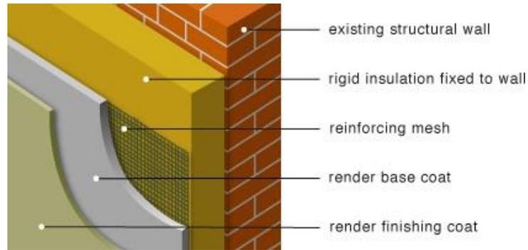
Fig 6. External wall insulation refers to the application of a wet render system onto an existing solid masonry wall. (Source: [www.greenspec.co.uk](http://www.greenspec.co.uk) building design), (Chinazzo, 2013-14)
