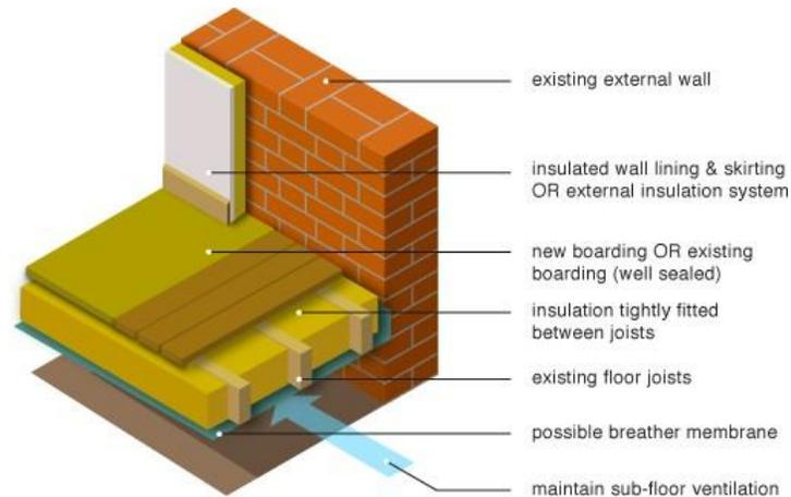
Fig 11. Timber ground floor insulation (Source: [www.greenspec.co.uk](http://www.greenspec.co.uk) buildingdesign).
