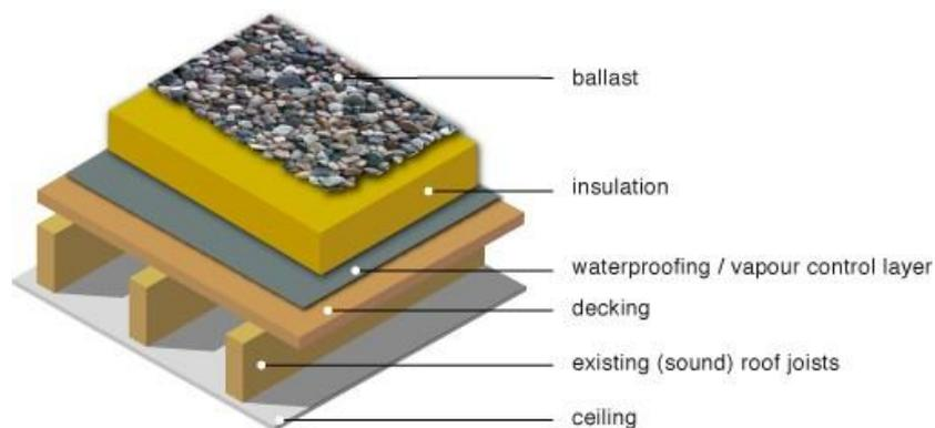
Fig 17. Inverted warm roof insulation (Source: [www.greenspec.co.uk](http://www.greenspec.co.uk) buildingdesign).
