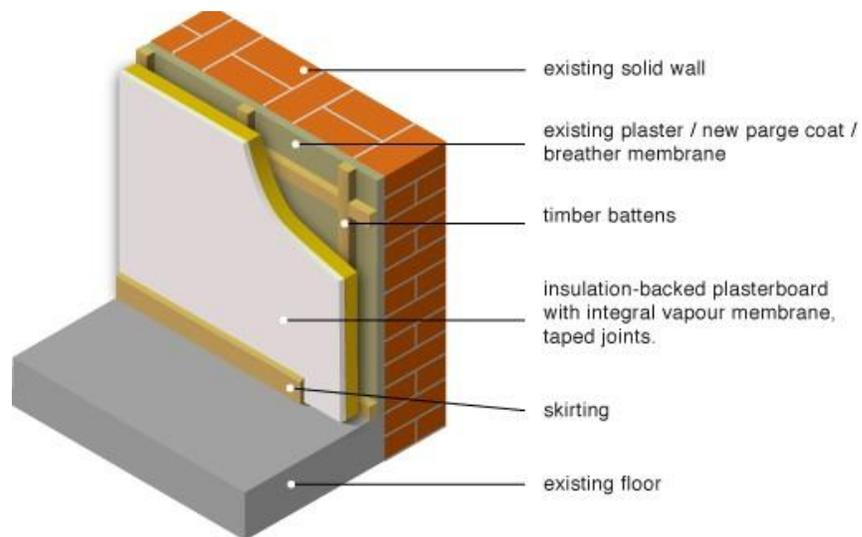
Fig 9. Internal wall insulation: battens with insulation (Source: [www.greenspec.co.uk](http://www.greenspec.co.uk) building design).
