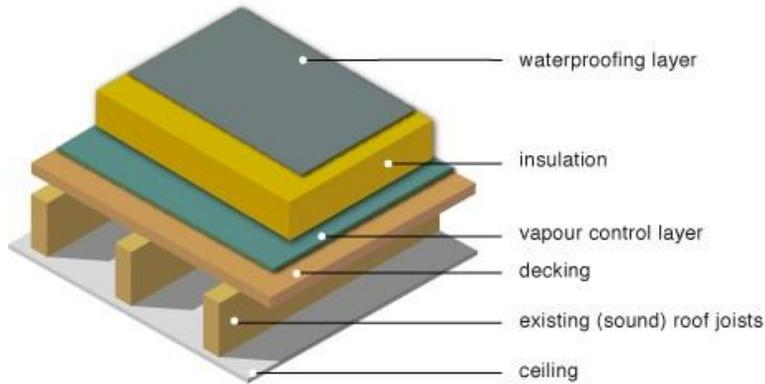
Fig 16. arm roof insulation (Source: [www.greenspec.co.uk](http://www.greenspec.co.uk) building design).
