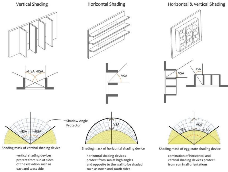
Fig 26. Shading performance. (Source: www.nzeb.in)
