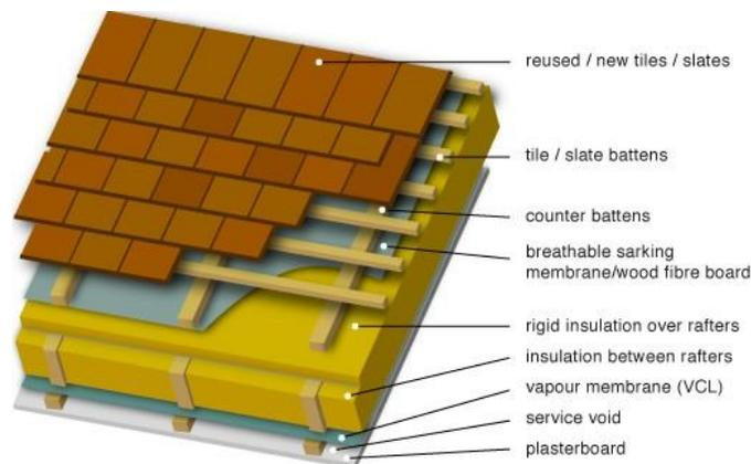
Fig 14. Roof insulation placed between and above the rafters. (Source: www.greenspec. co.uk building design), (Chinazzo, 2013-14)
