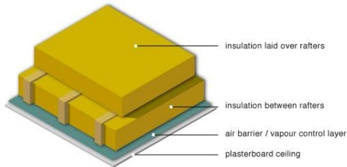
Fig 15. Loft insulation (Source: [www.greenspec.co.uk](http://www.greenspec.co.uk) building design).
