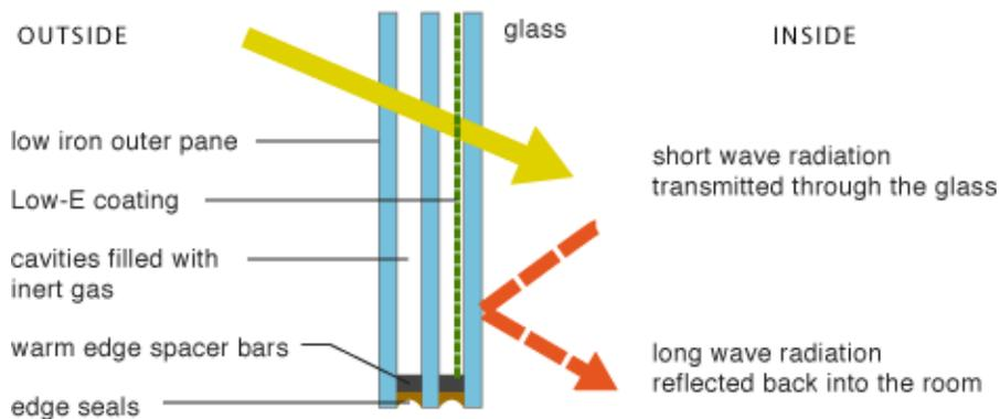
Fig 21. Low-Energy glazing (Source: [www.greenspec.co.uk](http://www.greenspec.co.uk) building design).
