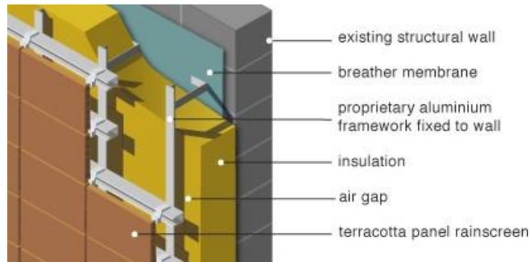
Fig 7. External wall insulation refers to a common method of applying a dry cladding system to an existing solid masonry wall. (Source: [www.greenspec.co.uk](http://www.greenspec.co.uk) building design), (Chinazzo, 2013-14)
