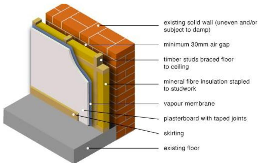
Fig 10. Insulating internal walls using studs and an air gap. (Source: [www.greenspec.co.uk](http://www.greenspec.co.uk) building design), (Chinazzo, 2013-14)
