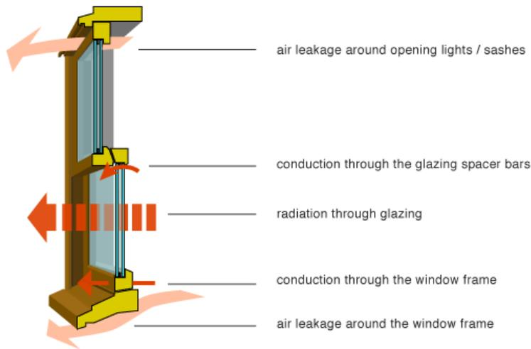
Fig 19. Heat losses through windows (Source: [www.greenspec.co.uk buildingdesign](http://www.greenspec.co.uk/buildingdesign/)).
