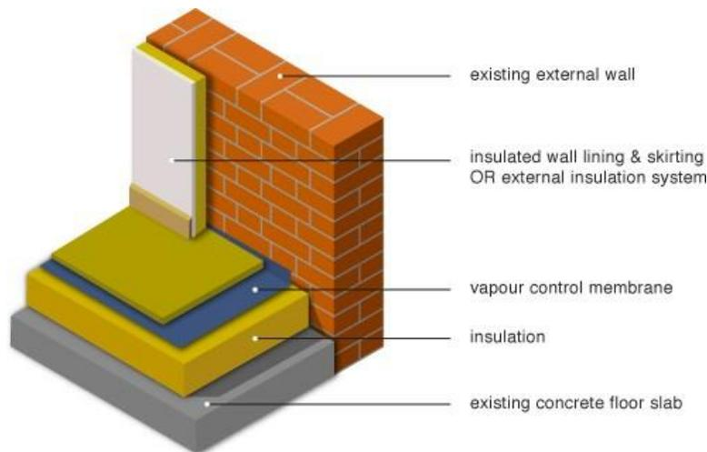
Fig 12. Concrete ground floor insulation (Source: [www.greenspec.co.uk](http://www.greenspec.co.uk) building design). (Chinazzo, 2013-14)
