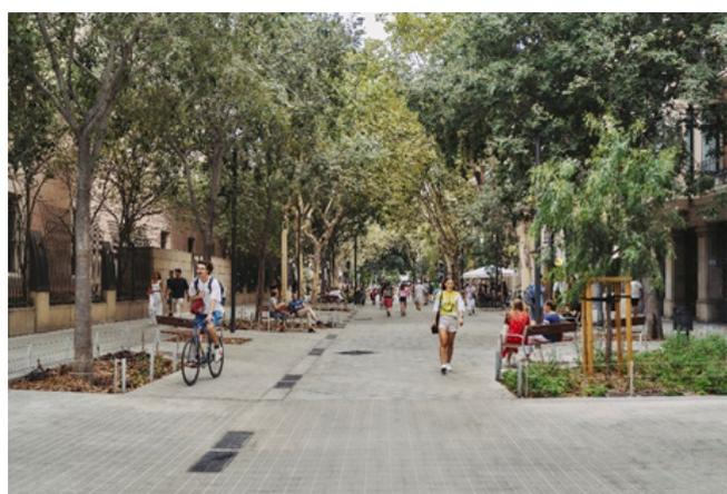
Figure 28. An example of an implemented green axis. The central portion of the street is shared among all users, while the two lateral strips, at the same level, are reserved to pedestrians. New planted areas are added and the asphalt is replaced with permeable paving (<https://www.urbidermis.com/es/blog/los-ejes-verdes-evolucionan-el-imaginario-urbano-de-barcelona/>)
