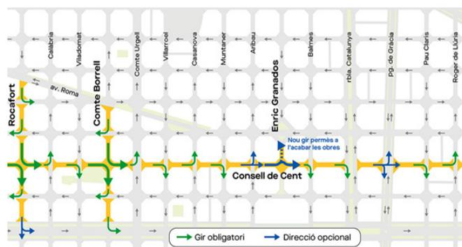
Figure 30. The circulation scheme along the green axis diverts through traffic on alternative streets, through street closures at intersections (Ajuntament de Barcelona, 2022b)
