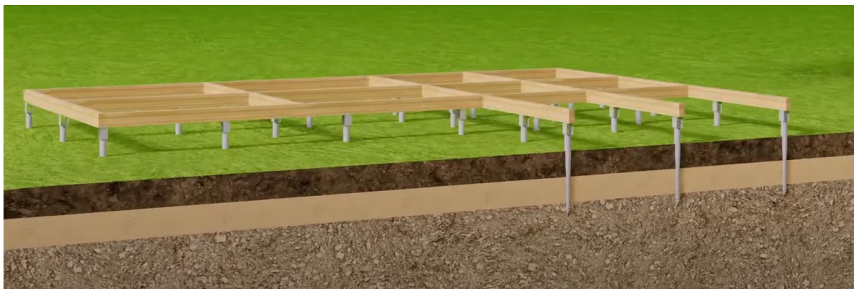
Figure 37: Ground Screws Foundation Illustration [99]
