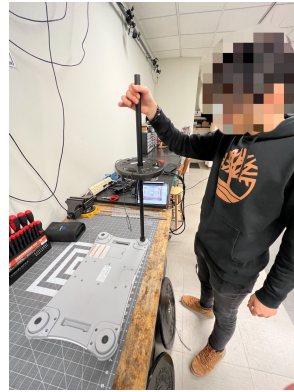
Figure 13: Weight application device and weights Figure 14: Load application method
