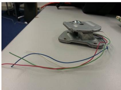
Figure 10: Extracted pressure sensor. Credits: <https://electronics.stackexchange.com/questions/83861/connect-wii-balanceboard-pressure-sensor-to-an-arduino>
