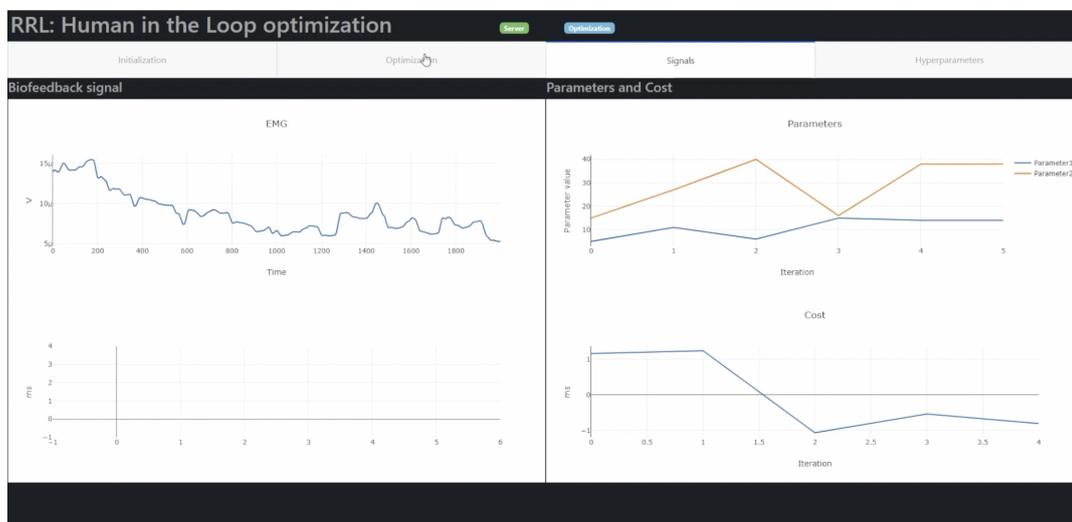
Figure 41: Signal tab from Optimization UI adapted to EMG optimization. Screenshot taken during the experiment.
