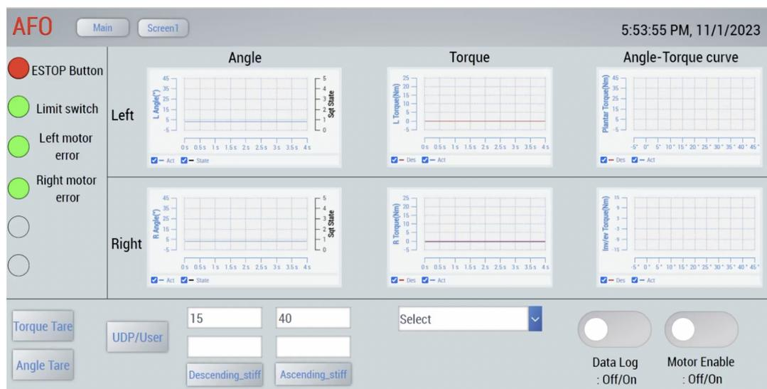
Figure 33: Control System User Interface
