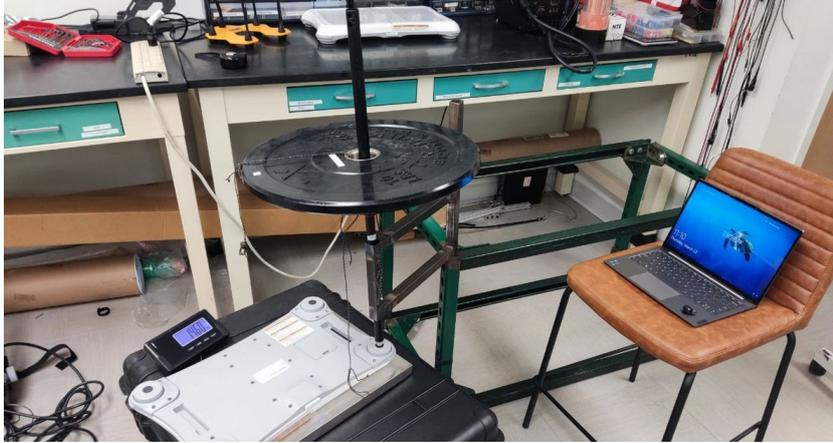
Figure 19: Setup for NewtonTransform calibration
