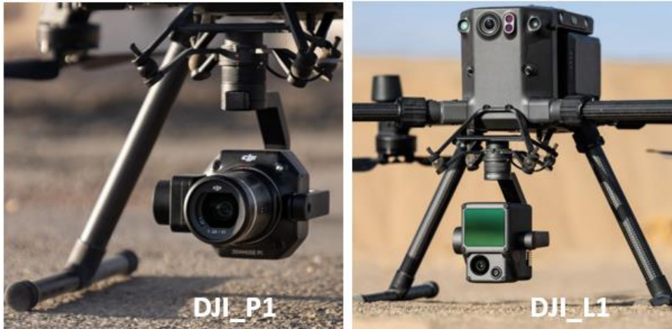
Figure 15. DJI_P1 and DJI_L1 sensors, mounted on the DJI M300 RTK drone, respectively, for photogrammetric and LiDAR flight.
