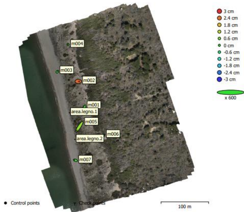
Fig. 3. GCP locations and error estimates. Z error is represented by ellipse color. X,Y errors are represented by ellipse shape. Estimated GCP locations are marked with a dot or crossing.
