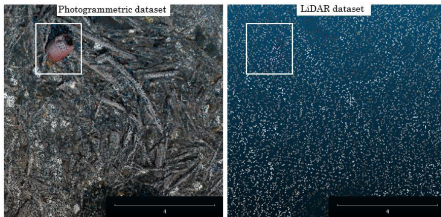
Figure 21. Photogrammetric and LiDAR point cloud densities comparison.
