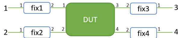
Figure 1.39: DUT with four ports.
