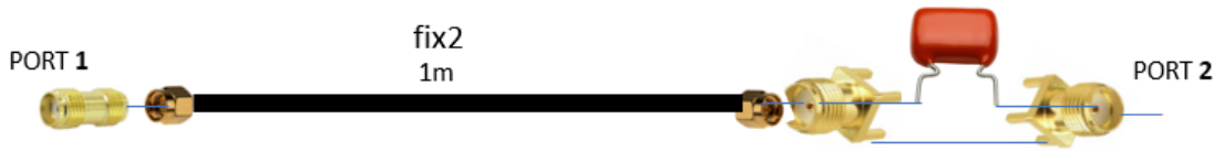
Figure 2.14: Schematic representation of the thru between fixture "1" and the capacitor.
