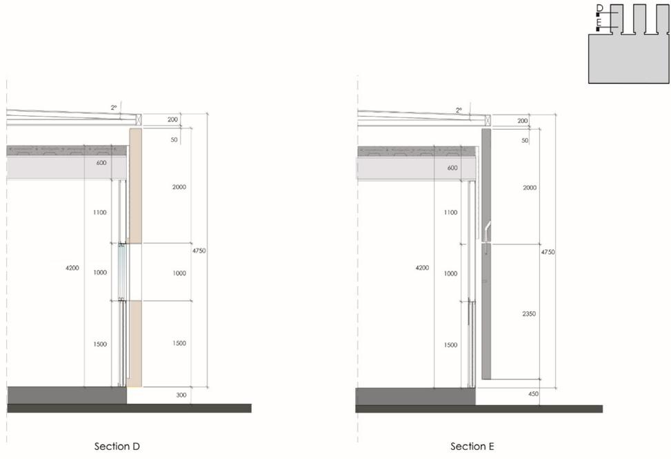
The façade of the wards was design with the modular system requirements, and were reduced to only two typologies, a full closed façade, and a window unit façade, using the same materials as the main body of the hospital so the design line was continuing even the construction system have changed.
