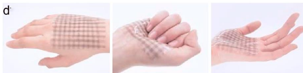
Figure 7 Demonstration of good adhesion and adaptation of the device when placed on a non-linear surface [9]
