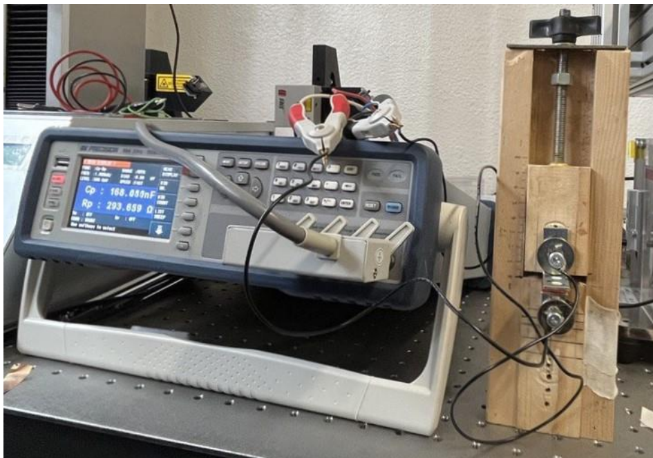
Figure 33 Set-up conductivity test over time.
