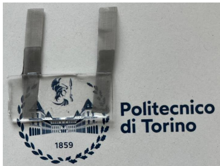
Figure 30 Tactile sensor final result
