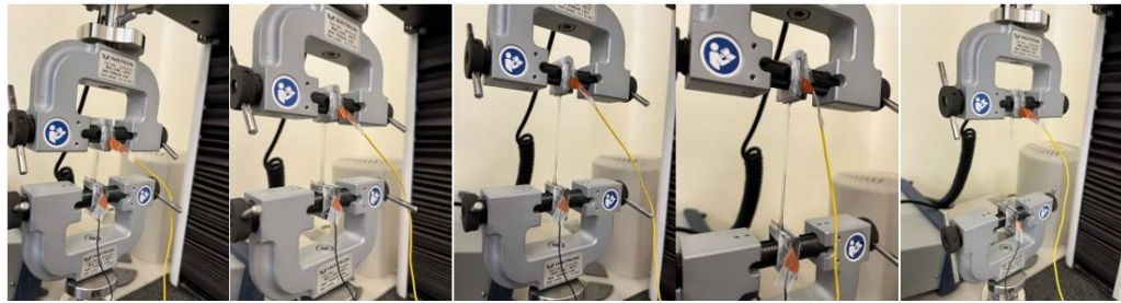
Figure 32 Different phases of a tensile test in which the sample is stretched to failure.
