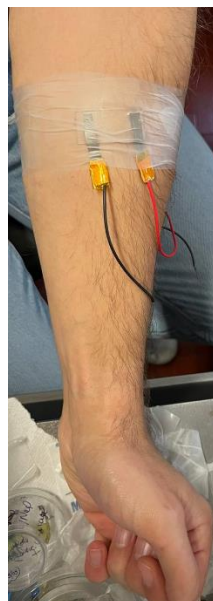
Figure 54 Test to check the sensor's ability to detect small deformations such as the movement of the hand flexor muscles.
