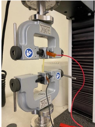
Figure 3.11. Assembly for tensile tests using dog bone shaped samples.
