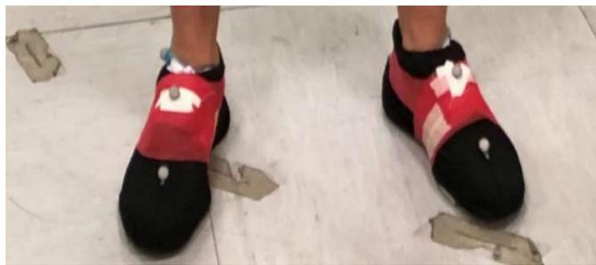
**Figure 3.1:** *Subject wearing an inertial sensor on the instep of each shoe, below the red tape, and retro-reflective markers.*
