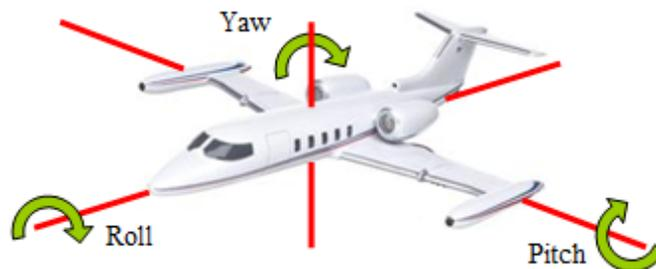
**Figure 1.12:** Representation of Yaw, Pitch and Roll. Adapted from [24].
