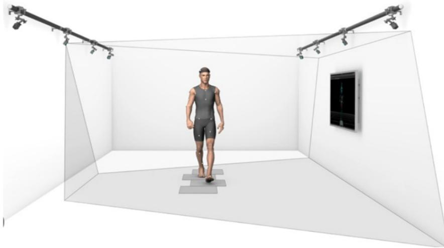
**Figure 1.5:** *Illustration of an Optoelectronic system.*
