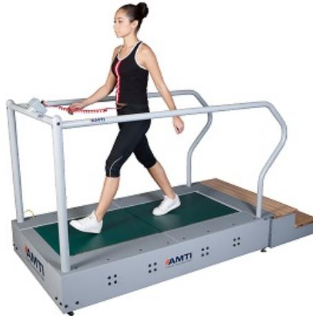
**Figure 1.7:** *Instrumented treadmill.*
