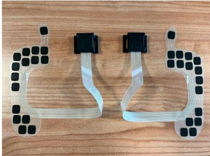
**Figure 1.15:** *Pressure Insoles from the INDIP system [32].*
