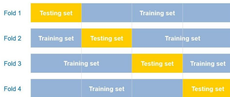
Figure 21: 4-fold cross-validation; each portion of the dataset is used as testing set once, while the rest constitutes the training set.
