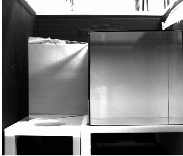
Figure 8.5: Image of the chosen setup. The scintillator and mirror are placed at 720 mm distance from the sensor. Graph paper was used to evaluate the position of the mirror.
