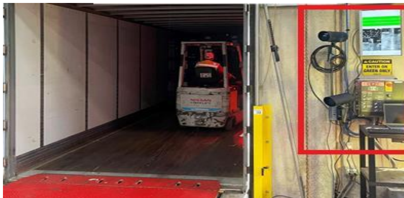
Figure 18. Camera scanning drive thru.
