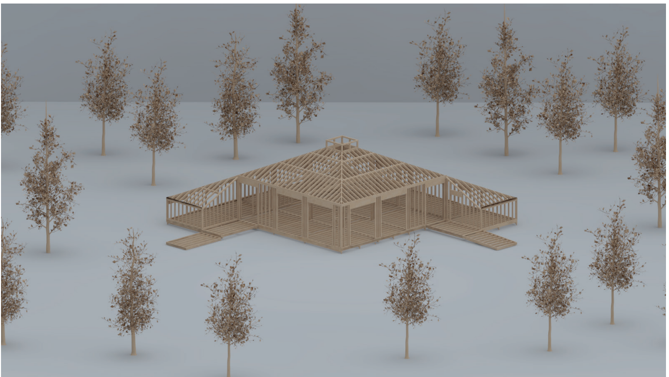
Figure 17 Construction Stage 4, addition of roof frame
