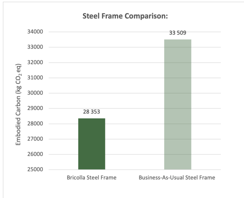
Figure 140: Embodied Carbon of the Bricolla and Business-As-Usual Case Steel Frame. Reference: Author.
