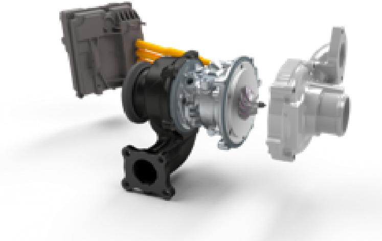
**Figure 2.5:** E-Turbocharger with dedicated control unit
