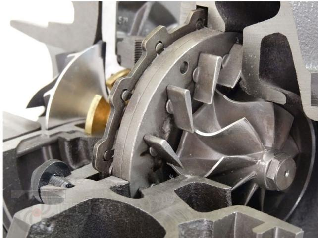
**Figure 2.4:** Turbocharger with VNT system[20]
