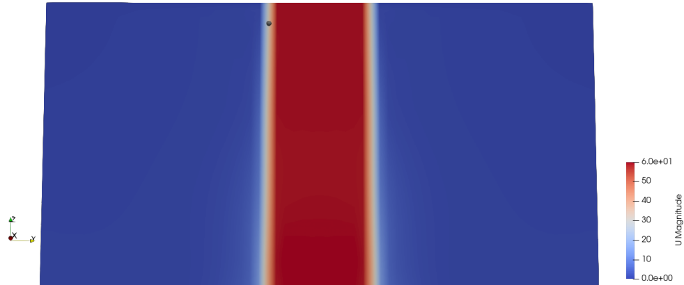
Figure 3.2: Visualizing the airflow and droplet injection location for Case 2.
