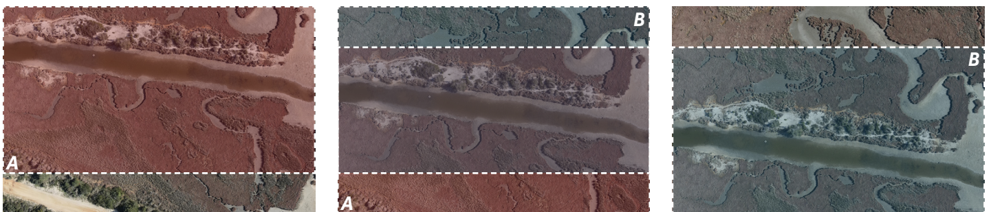
Three photos displaying "overlap" of similar features - 80% overlap between two successive photos
