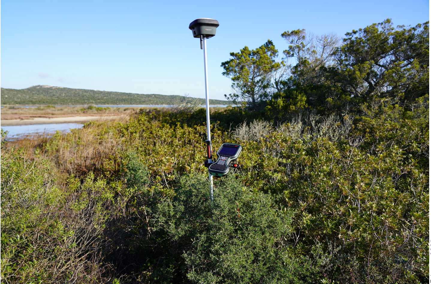
"Leica CS20 Field Controller" (below) e "Leica GS18 GNSS RTK Rover" (above) with tilt error correction technology 7 - geolocating plant species
