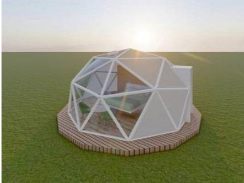
Figure 29 – Geodesic Domes Shelter exterior view number01
