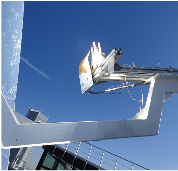
Figure 7.12: White SiC sample installed in the solar dish system
