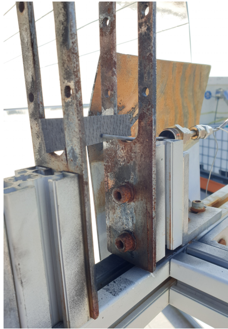
Figure 7.19: Black SiC sample and thermocouple for the measurement of temperature
