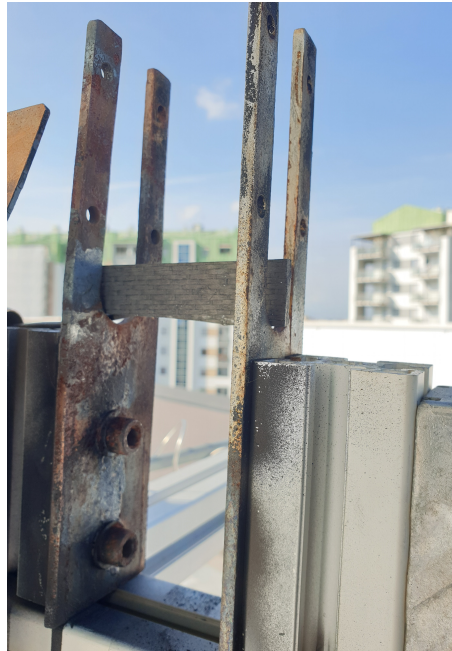
Figure 7.18: Black SiC sample installed in the receiver support
