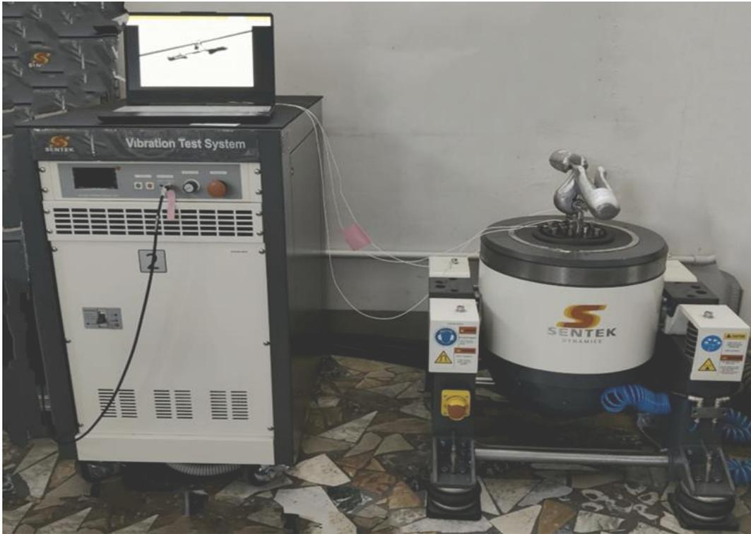
**Figure 2.3.** Experimental setup for Stockbridge analysis (Lab)
