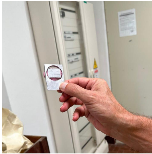
Figure 42: Sample holder using polymer clay for XRD machine.
