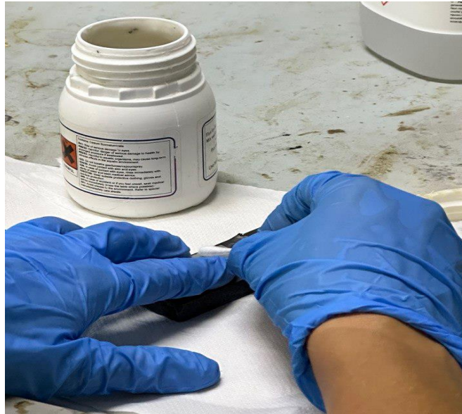
Figure 50: Application of flux on aluminum
