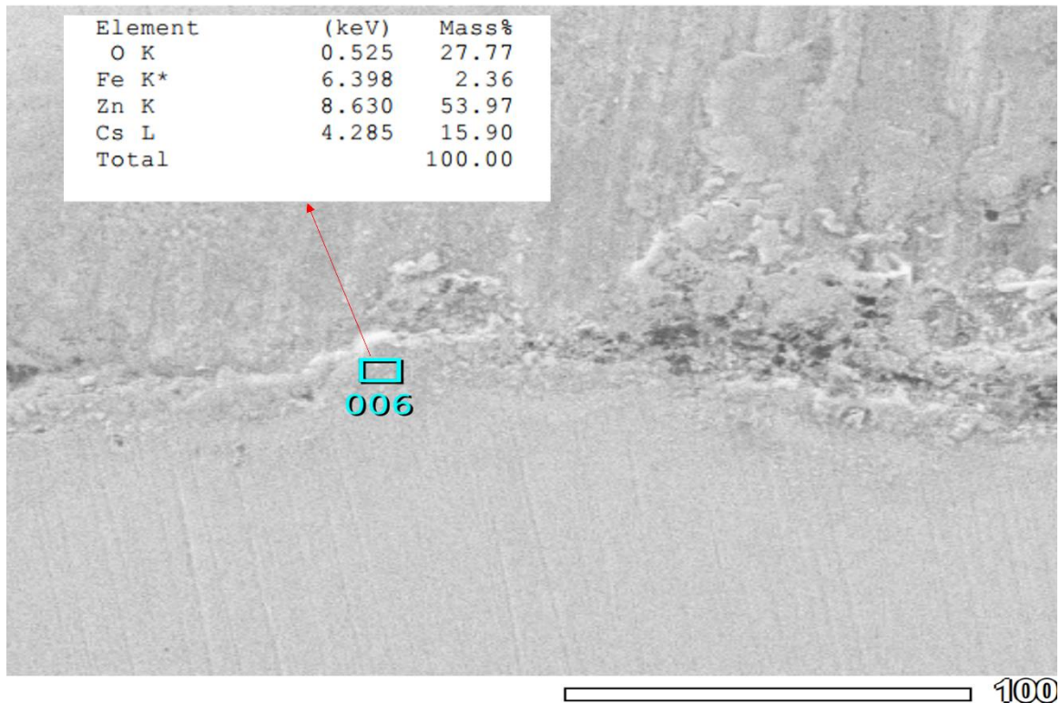
Figure 81: SEM-EDS analysis of joining area of traversal cross section of sample with flux showing local chemical composition on interface layer between Steel and Zn.
