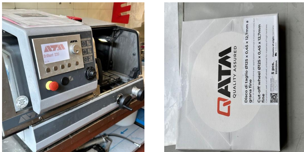
Figure 38: Cutting machine and alumina blade.
