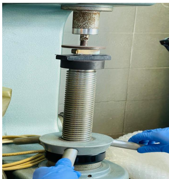
Figure 52: Pressing of Stack with Mechanical Presser
