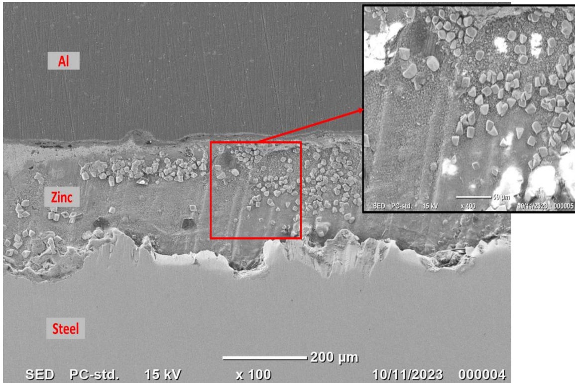
Figure 75: SEM-EDS analysis of joining area of traversal cross section of sample with flux.
