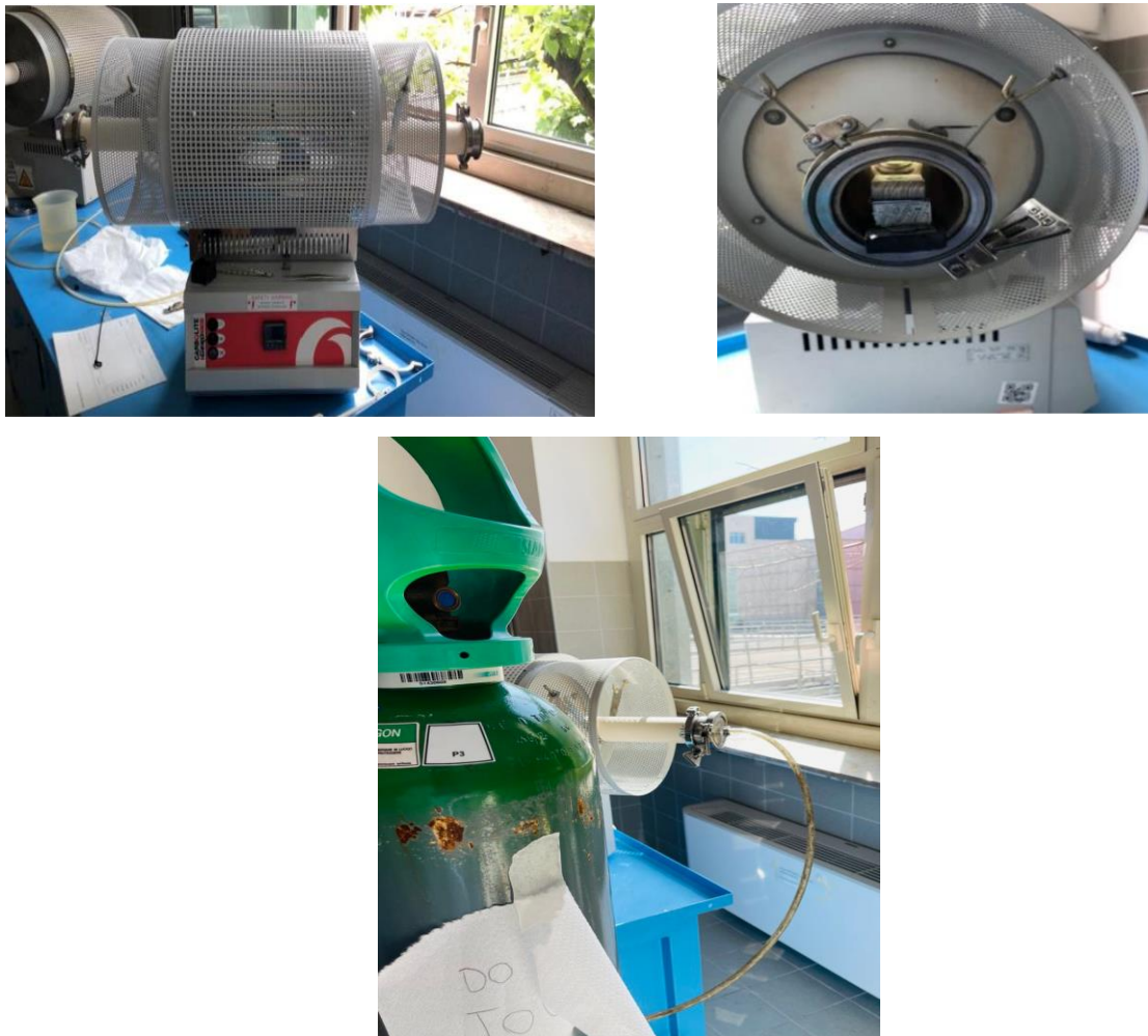
Figure 53: Tubular Furnace with attachment to Argon cylinder
