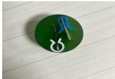
Figure 69: Resin mounting and polishing of traverse cross section of failed sample
