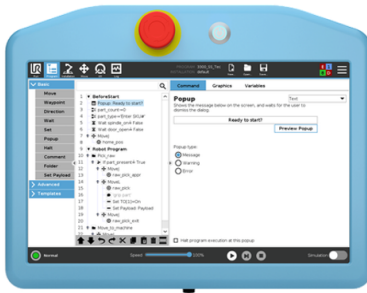
Figure A.2: UR3e teach pendant, picture taken from [41]
