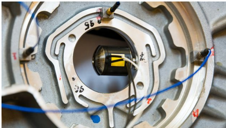
Figure 1.6: Miniature shaker for automotive NVH testing [11].
