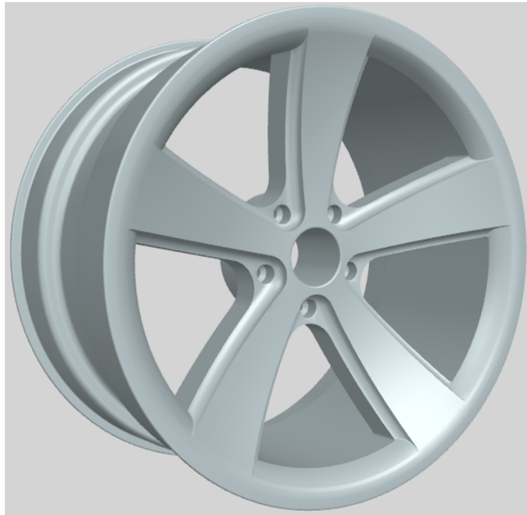
Figure 3.7: 3D model of the BMW 128 rim.
