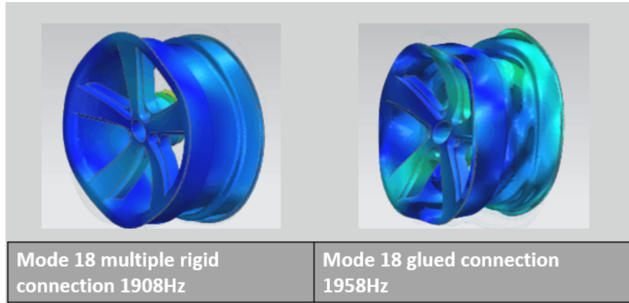
Figure 5.12: Mode 18 – th for the multiple and glued connections, input load F_z .
