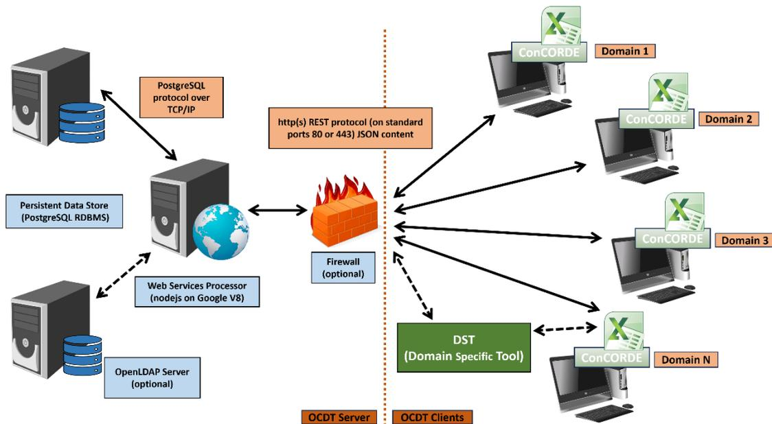
Figure 4: Schematic Overview of the OCDT architecture
