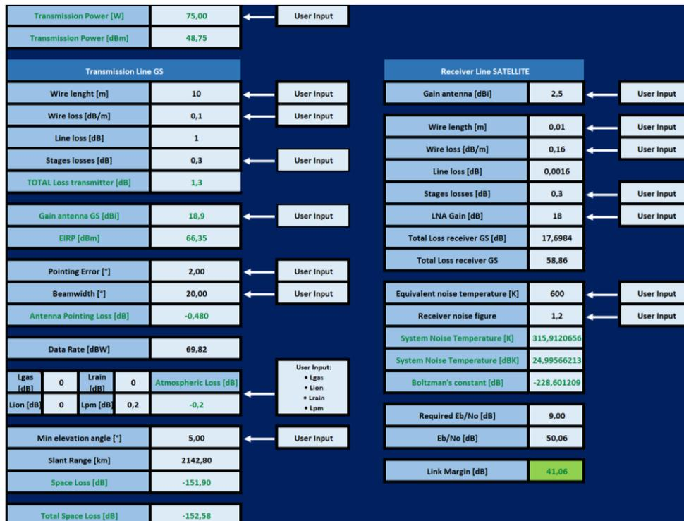
Figure 40: Spei Satellites Uplink Tool Output
