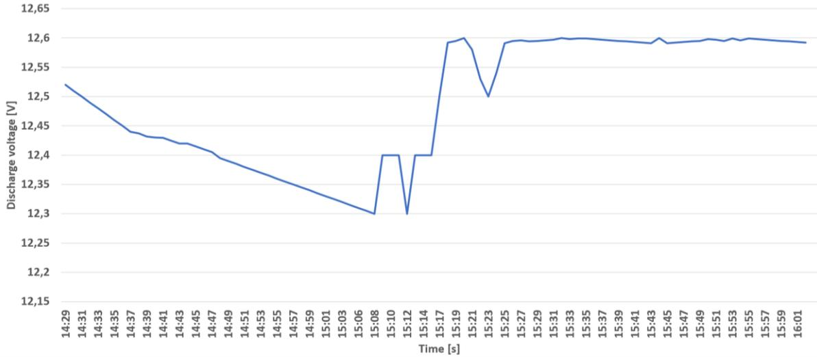
Figure 43: Spei Satellites Discharge Voltage
