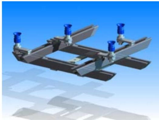
**Figure 2.13:** Reconfigurable gripper for plastic part extraction proposed in [5]
