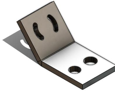
**Figure 5.41:** Provisional bracket for piece detecting sensor
