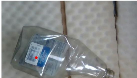
**Figure 7.14:** Example of a scene view with a transparent bottle, the red point indicates the grasp point predicted by the neural network.
