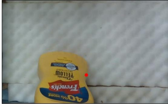
**Figure 7.8:** Example of a scene view with a detergent bottle, the red point indicates the grasp point predicted by the neural network.
