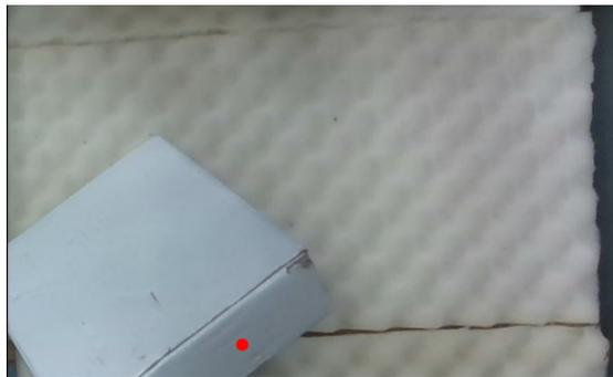
**Figure 7.9:** Example of a scene view with a box, the red point indicates the grasp point predicted by the neural network.
