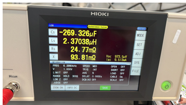
FIGURE 6.25: Impedance of the negative cable for the connection to the active load.
