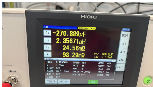
FIGURE 6.24: Impedance of the positive cable for the connection to the active load.
