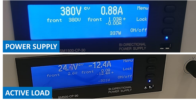
FIGURE 6.23: Display of the power supply and active load in the nominal conditions.
