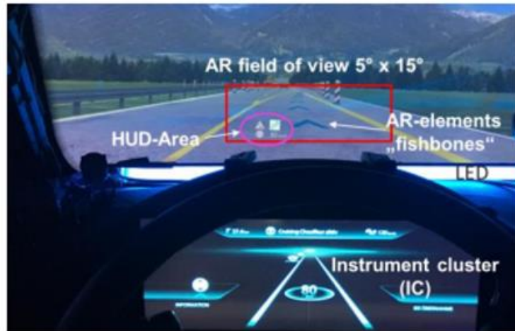
Figure 24 - Overview of HMI elements used in the simulator study from [20]
