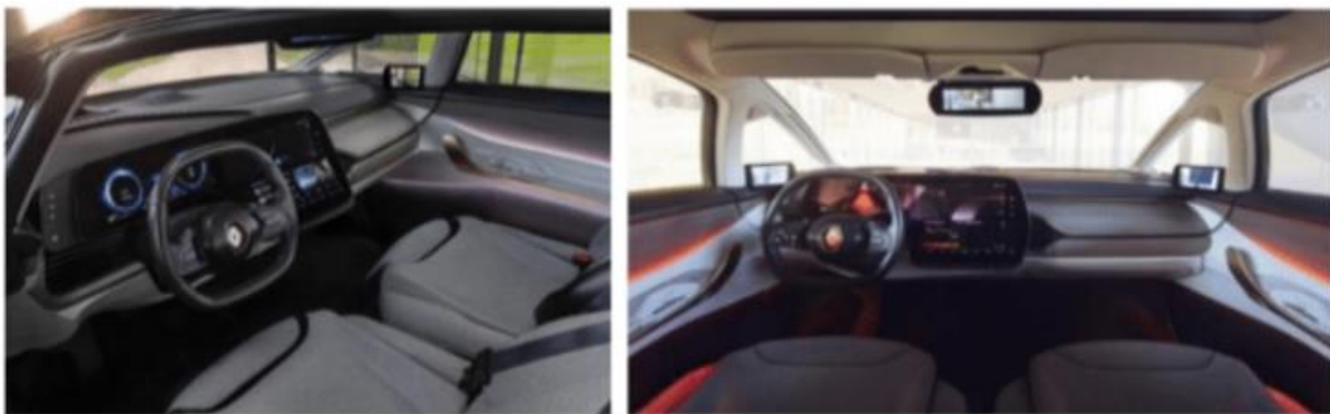
Figure 19 - SYMBIOZ demo car cockpit from [14]. When ambient light and HMI become orange, AD mode is activated
