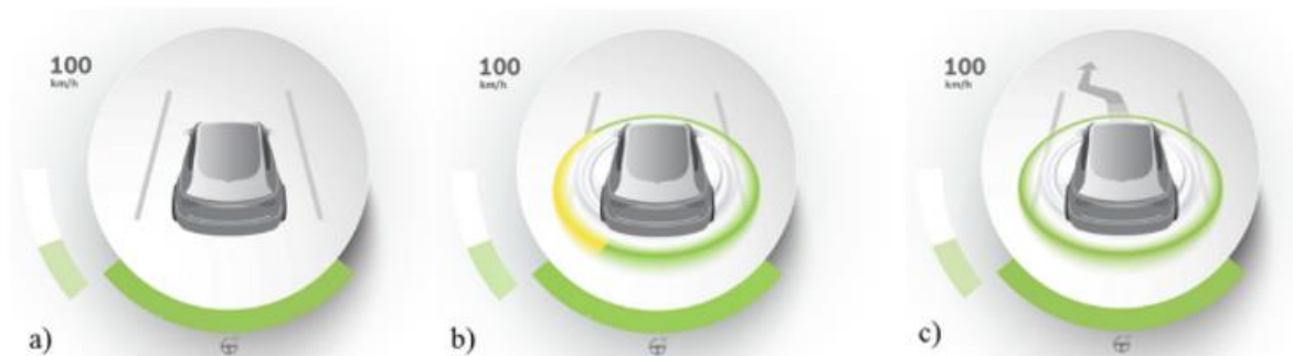
Figure 9 - Cluster's level of feedback from [3]. (a) No feedback; (b) Sensors feedback; (c) Sensors and
