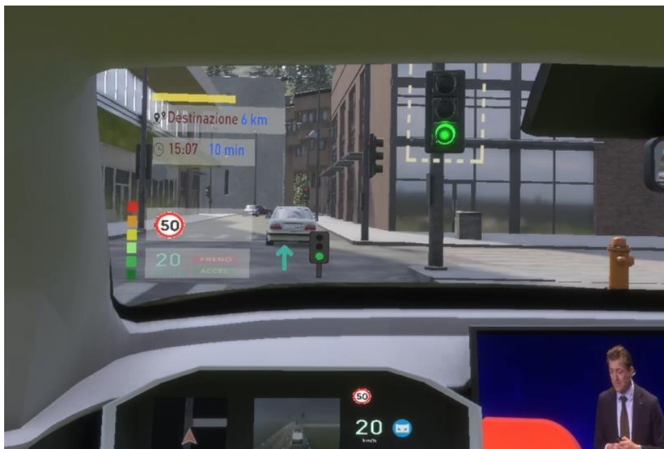
Figure 69 - Windshield display screen fixed information and AR detection box
