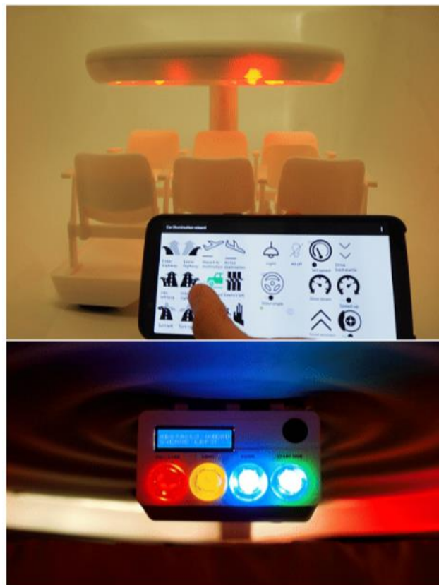
Figure 21 - On top, prototyping platform with wizard interface on a smartphone. On bottom, control unit inside the car prototype with lit-up buttons from [15]
