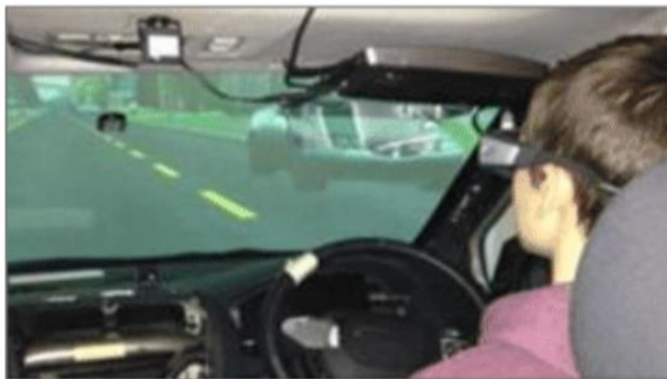
Figure 33 - In-vehicle setup showing the HUD, road scene and participant wearing ETG from [27]
