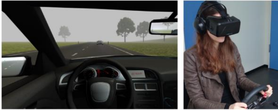
Figure 35 - Left: a car approaching out of the fog (visual range: 200m) ahead of the driving car. Right: virtual reality study setup using Oculus Rift DK2. From [32]
