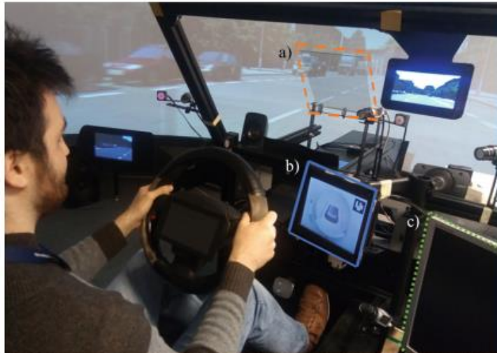
Figure 8 - (a) Head-up display (orange dashed outline); (b) Assistive cluster interface (blue solid outline); (c) Touchscreen display (green dotted outline) used in [3]
