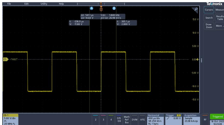
**Figure 5.6:** Channel 1 (yellow line) shows the PWM generated by EVSE in D state.
