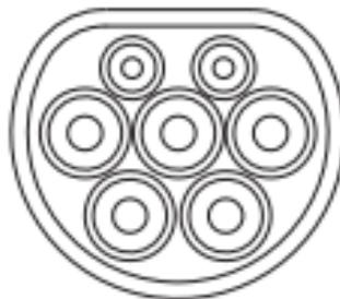
**Figure 2.3:** Connector Type 2 with 7 contacts [3]
