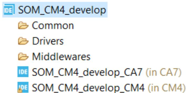
**Figure 4.3:** Project folders created by STM32CubeMX after code generation
